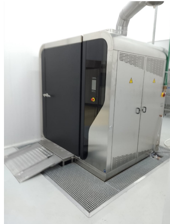
Pit mounted w/ramps
