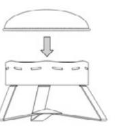
A steel mesh safety cover is included with all EcoServes and should be placed over the hotplate when no dish is covering the exposed hotplate.
